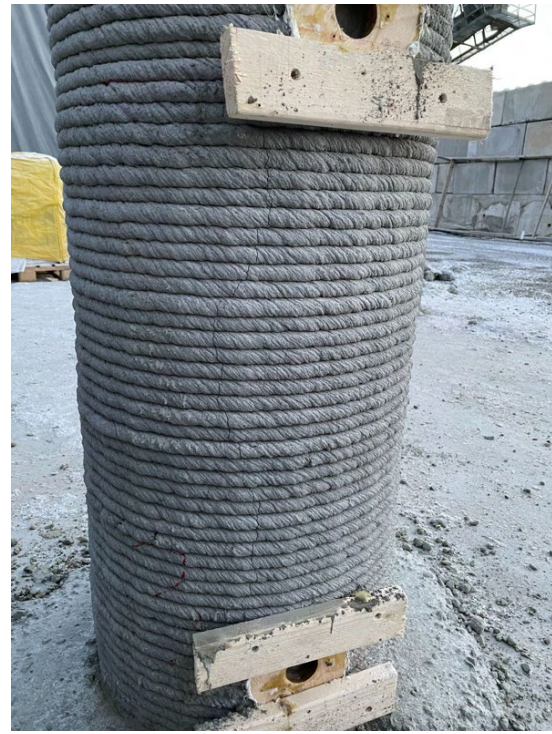
Figur 8: Fina, vertikala sprickor i formarna p.g.a. temperatureffekter. (Shabo & Hossein, 2022).
