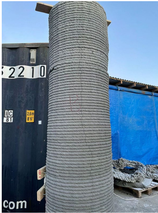
Figur 8: Fina, vertikala sprickor i formarna p.g.a. temperatureffekter. (Shabo & Hossein, 2022).
